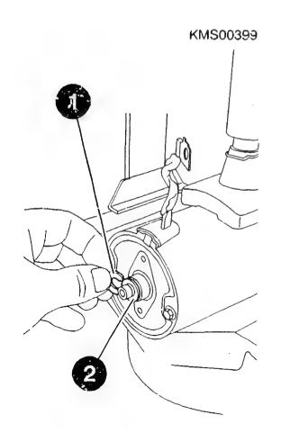
Disassembling commutator end shield
